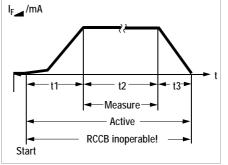
The test instrument generates a DC residual current which saturates the magnetic circuit of the RCCB. The PROF/TEST®C superimposes a measuring current which demonstrates only half-waves of like polarity. The RCCB cannot detect
